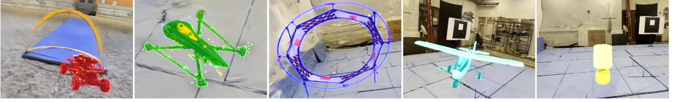
Fig. 3: Automatically Labeled Synthetic Data: FalconApp renders synthetic images with render-aligned masks for objects with diverse geometry and appearance.
